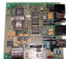
Base Station Controller including phone patch & repeater controller
